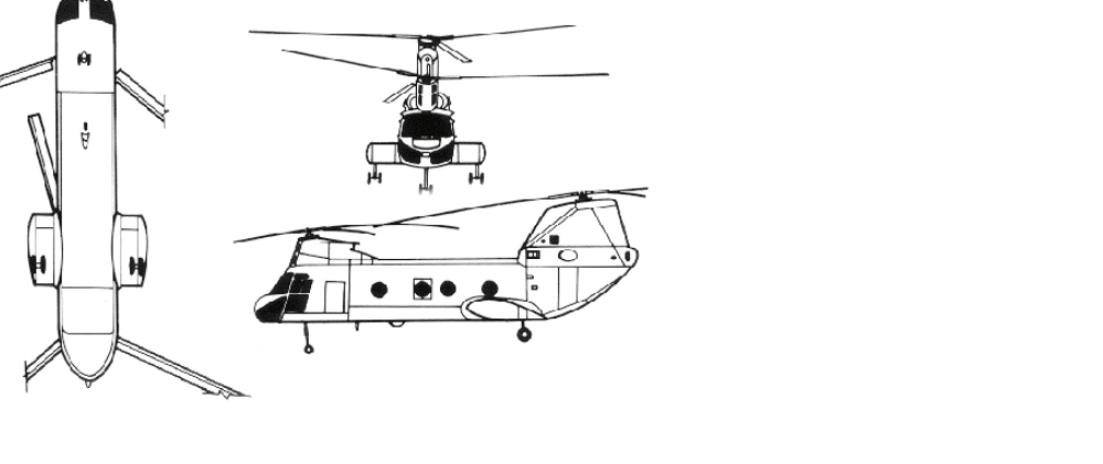
BOEING VERTOL CH-47 CHINOOK Rotor Diameter = 60 ft Length = 52 ft Gross Weight = 50,000 lb UL = 24,000 lbs
