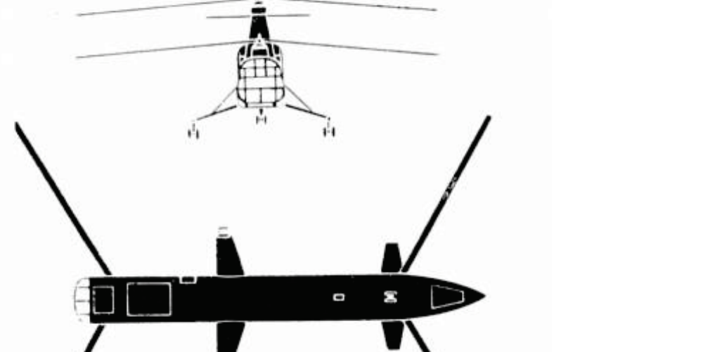
Boeing XCH-62 HX Rotor Diameter = 92 ft Length = 87.2 ft Gross Weight = 118,000 lb UL = 58,420 lbs
